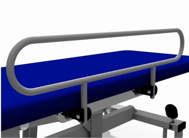
**To raise the cot side** from the down position; lift and rotate the cot side towards you through a full 180°. When upright push the cot side down into the plastic block until it is fully located.
