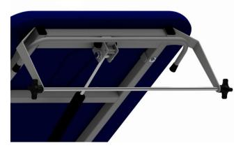
Paper roll is replaced by removal of one or the other of the plastic knobs, sliding the bar partially through the leg of the holder and then fitting the tube over the bar. Re fit in the reverse order.
